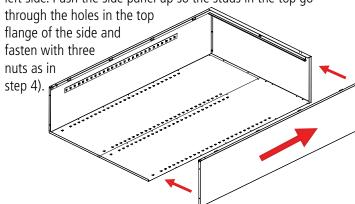
**6.** Attach the sill (Ref. No. 8) to the sides. Place nuts loosely on each of the studs and slide the ends of the sill into the slots on both sides of the unit. Then, securely tighten the nuts.
