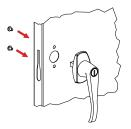
**1.** Place the locking handle (Ref. No. 12) on the right hand door and fasten with two #8-32 X <sup>1</sup>/4 hex-head bolts and lock washers, provided with the handle.
